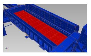
The shear lets you work in parallel or angular mode. With the powerful side compression block in the parallel position and the compression lid half closed, the scrap in the box is compressed as far as possible.
