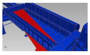
By changing the angled force to the opposite end of the piece will practically eliminate any resistance thereby fully compressing the material. The lid goes down, compressing the scrap downward beyond the final closed position of the lid. Then the lid is raised slightly above its final closed position. The side compression block is fully extended and the lid is finally closed. The log is now ready to be fed to the shear head.
