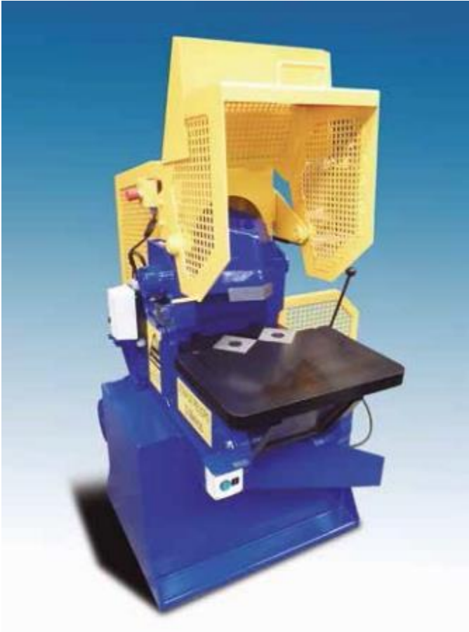
H-H-11 “Nutcracker” Special shear to clean non-ferrous materials.
